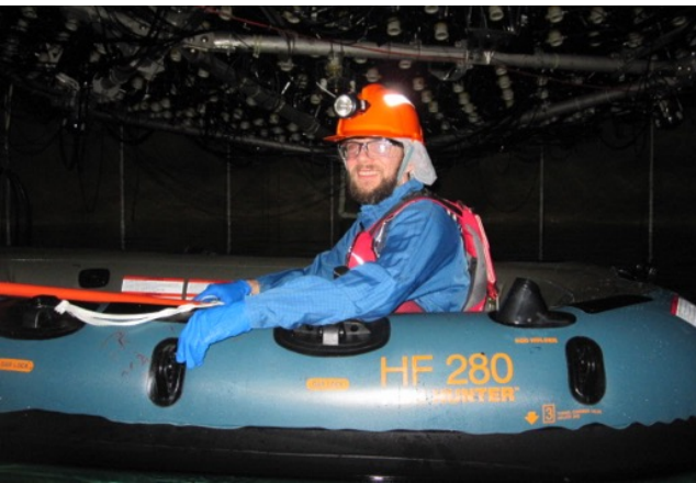
(above) Teal replacing PMTs in the SNO+ detector during commissioning
