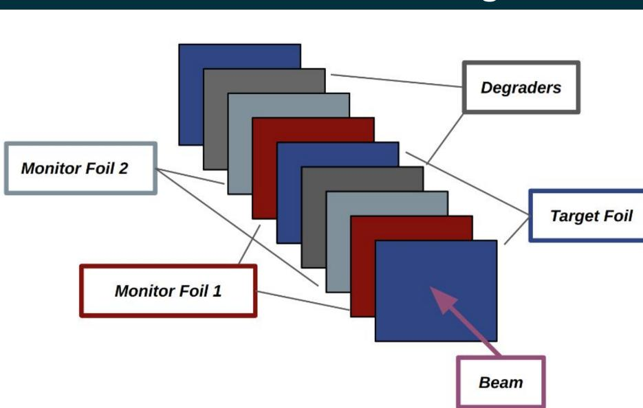
**Monitor foils (AI, Cu)** with known cross sections characterize the incident beam as it propagates through the target stack.
