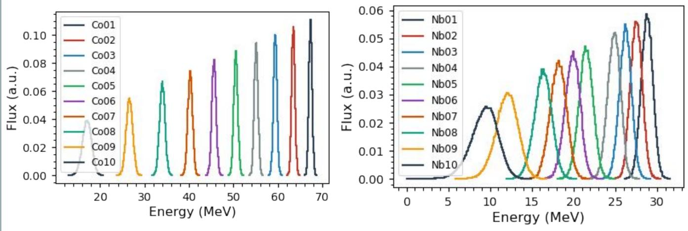
With the Curie python script developed by researchers at LBNL, we can model the entire stack of target foils, monitor foils, and degraders to plot the energy loss and flux through each of the target foils as the beam propagates through the stack. From this we can determine the number of degrader foils needed to ensure data points in the energy regions of interest.
