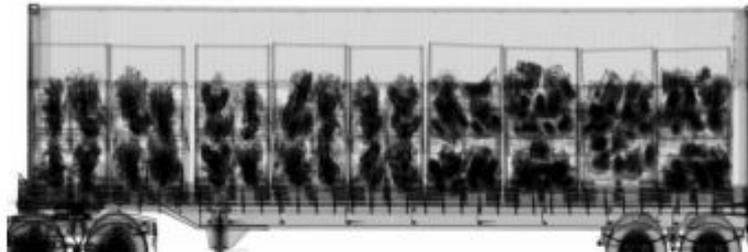
Fig. 3. Example cargo radiograph from a Smiths Detection HCVP NII system.
