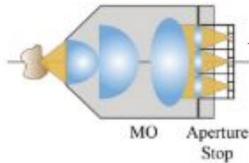
$N$  microlenses (in diagonal) subsample the aperture (of Fourier) plane of the microscope objective
