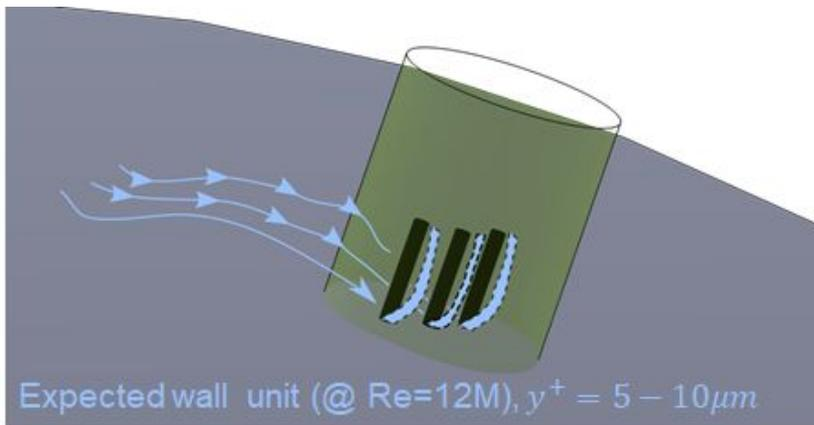
Tagged pattern (black) is deformed (blue) by the fluid flow
