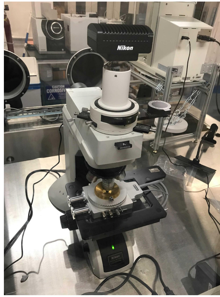
Left: Linkam Stage for high-temperature optical spectroscopy on optical microscope in SALT lab glovebox
