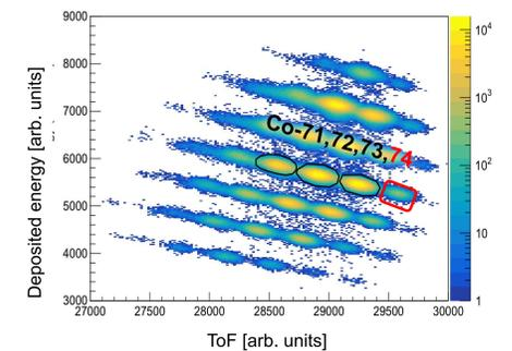
Fig. 11: Time of Flight spectra from the cocktail beam, where Co-isotopes have been circled in black or red. From Ref. [4]
