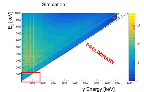
Fig. 10: Fit of simulation to extract I<sub>β</sub> for <sup>72</sup>Co. Note the area marked in red for β delayed neutron emission.
