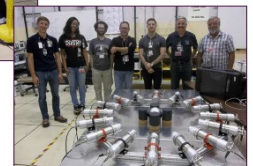
Right: Team of CNEC/CVT faculty, students and post-docs performing active measurements of correlated particle emissions from HEU pellets surrounded by americium-beryllium sources.
