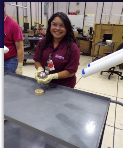
Student holding the BeRP Ball (4.5 kg sphere of \alpha -phase weapons-grade Pu) at the NCERC.
