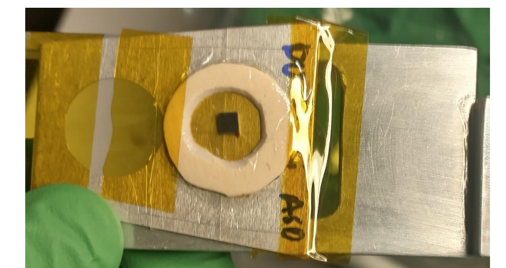
Fig 7. Uranium taggant monolith in containment system of polypropylene and Kapton.
