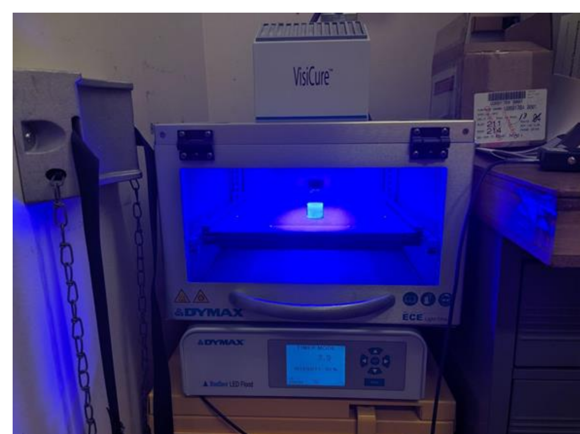
UV Curing in progress
