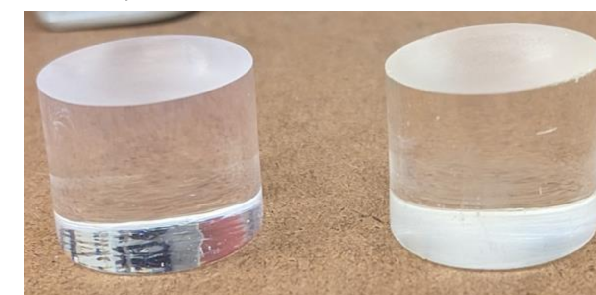
AFIT(left) and LBNL (right) scintillators after curing, sanding, and polishing
