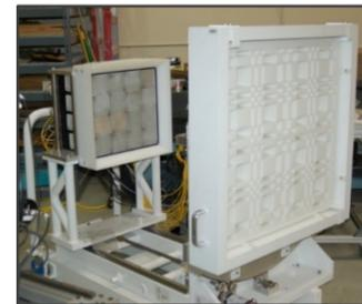
Neutron coded aperture imaging detector
